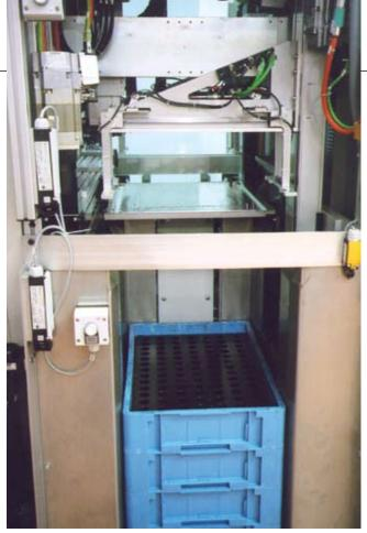
▲ More extensive post-process part handling is exemplified by this palletization system that is built into the machine tool. Finished parts can be first inspected automatically by a laser gage or other device, then loaded into a pallet. These flexible pallets can also be used to load uncut forgings or other chucked parts and receive the finished parts.
