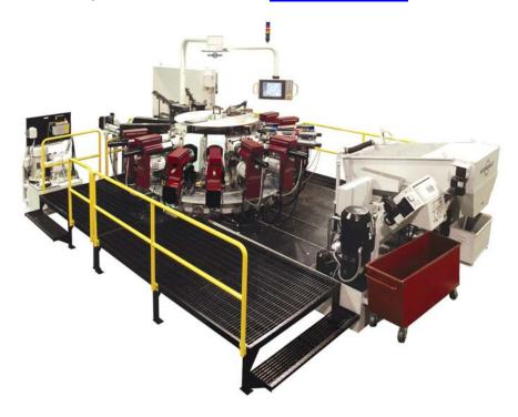
*Caption:* The Hydromat EPIC R/T HS 16 Indexing Chuck Rotary Transfer machines produce precision metalcutting for cast parts, near-net shapes, profiled stock and standard bars. It's designed with the flexibility and versatility to easily accommodate a variety of part families within it's 76 mm cube capacity.
