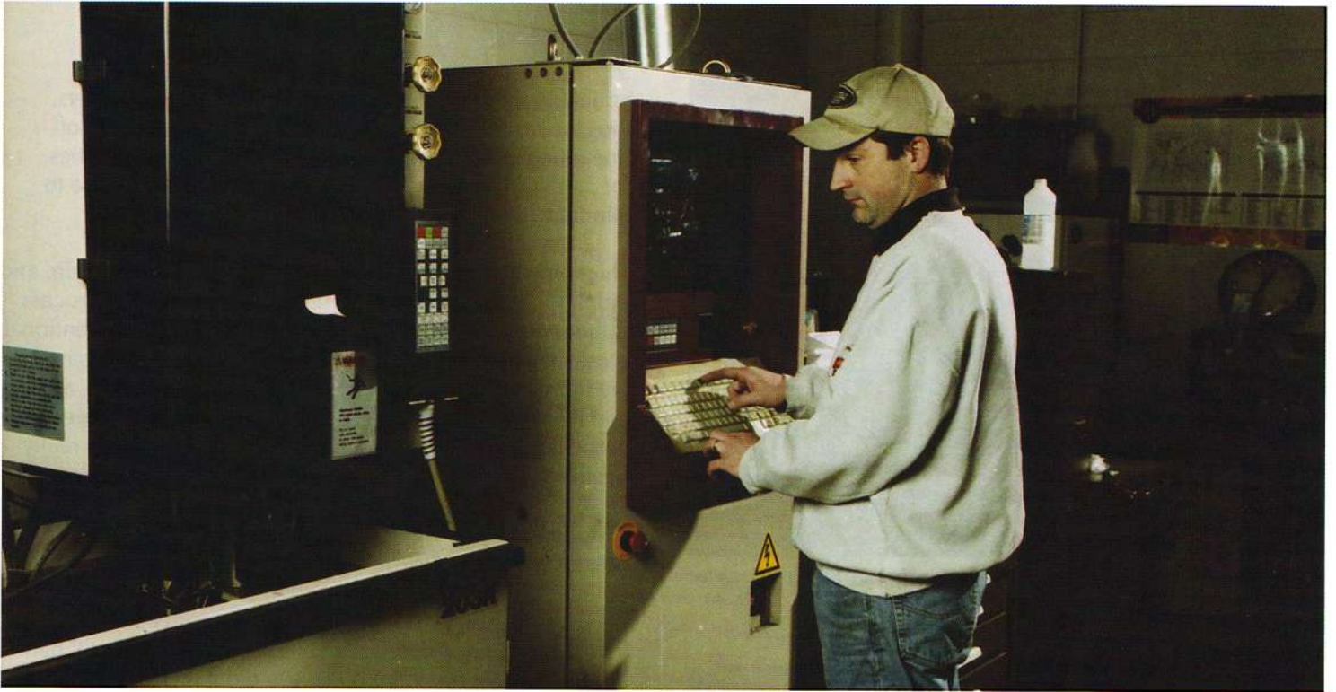
The purchase of a Hatachi Wire EDM (above) has given D&S an edge in manufacturing its own custom tooling. Grinding existing tooling now runs automatically on a Blanchard table grinder (below).
