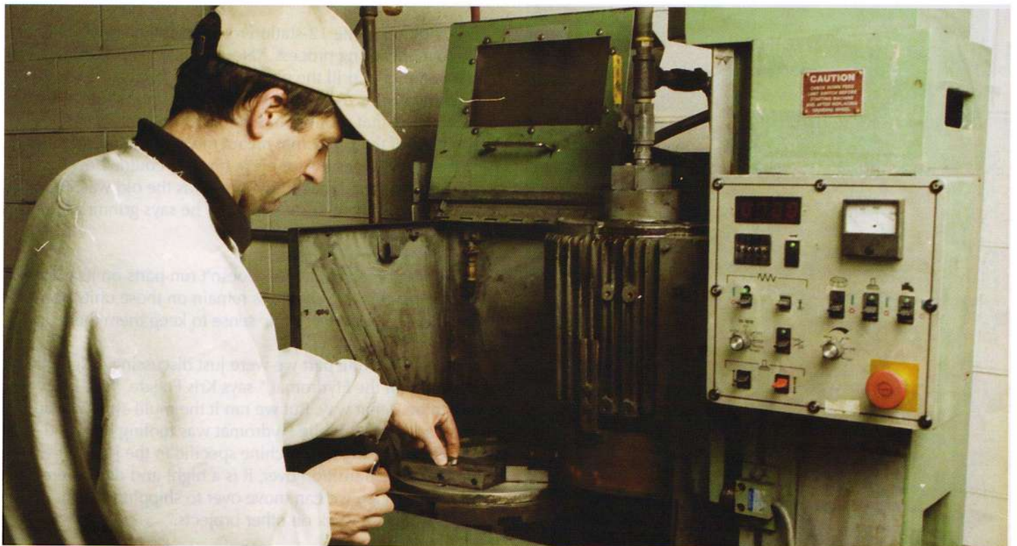
The purchase of a Hatachi Wire EDM (above) has given D&S an edge in manufacturing its own custom tooling. Grinding existing tooling now runs automatically on a Blanchard table grinder (below).
