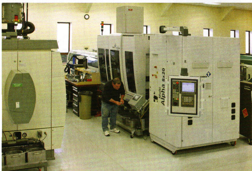
▲ The company's newest CNC multi-spindle is a Tornos Multi Alpha 8x20. With eight stations, it is able to machine more complex parts than the company's first CNC six-spindle machine.
