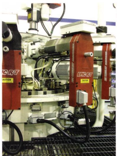
Each tool spindle unit carries its programmed motion instructions. These units can be moved from station to station as needed with no need to reconfigure the CNC except to tell it where the tool spindle unit is. Only four connections are needed for each tool spindle unit.
