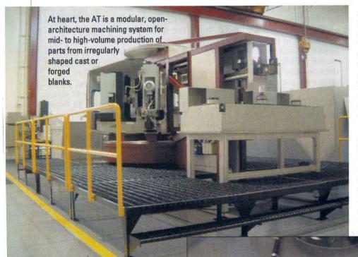
ccording to Martin Weber, Avice president, manufacturing, Hydromat Inc. (St. Louis), the company's new AT (Advanced Technology) rotary transfer machine departs from proven design and processing features of its machine type to create "an entirely new processing method, one that opens the door to a wide variety of new applications."
