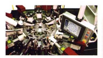
Systems have always had to justify the long changeover times of such machines by running high-volume jobs. But this is no longer the case because today's advanced rotary transfer machines changeover in hours, making them cost effective and competitive for low-volume jobshop environments as well.
